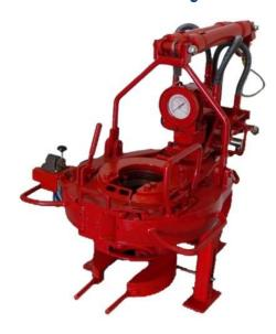
BVM Tongs are available in a variety of models, sizes and types to handle casings, drill collars, sucker rods and tubing tubulars and can be supplied with hydraulic or manual backup assemblies.
