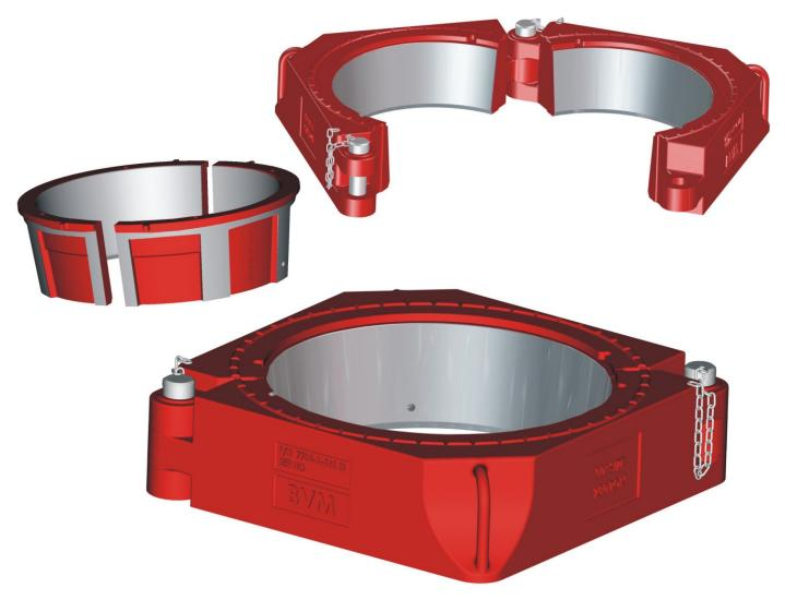
BVM Hinged casing spiders and bushings are well suited to use where casing needs to be run through a rotary table or where no rotary table is in place. They can sip on the rig floor or be supported by cribbing. With our range of sizes they can be used with most sizes of casing. All bores, except the internal bore of the 8.5/8", are 3" per foot tapers to use UC-3 or other 3" taper slips. The 8.5/8" is 4" per foot taper to be used with API standard smaller slips.
