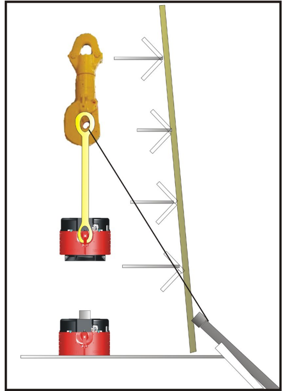
Figure 2-7. Standard Derrick Installation
