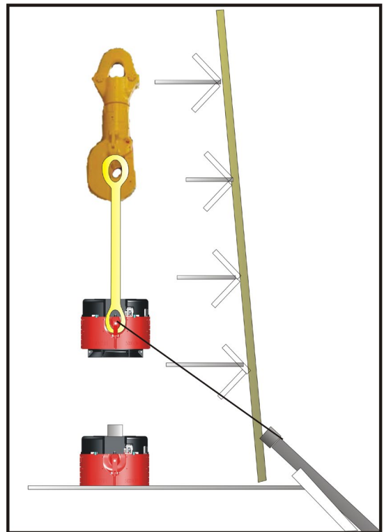
Figure 2-8. Jackknife Derrick Installation
