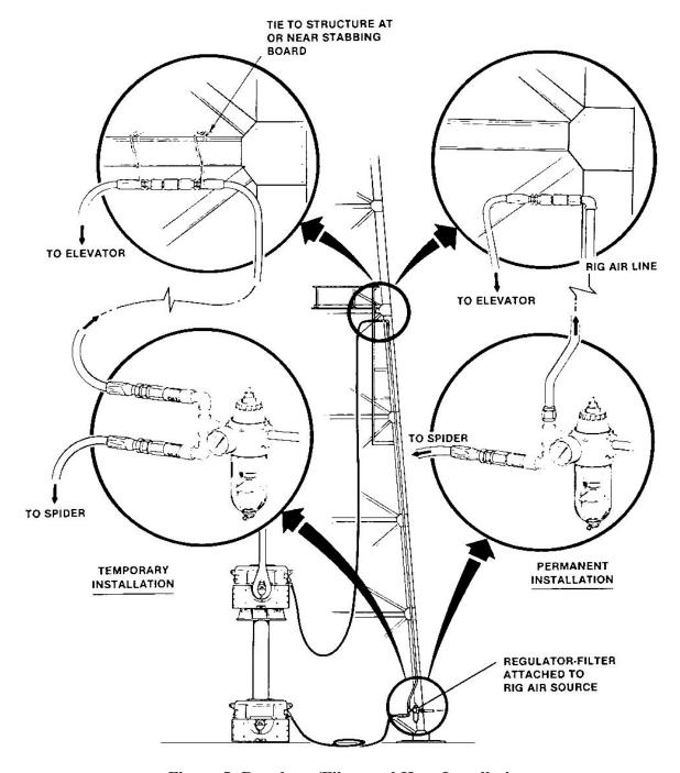
Figure 5: Regulator/Filter and Hose Installation
