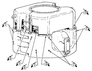
Figure 9: Lubrication points
