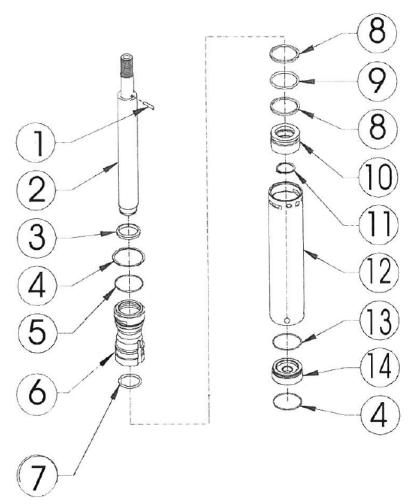
Figure 17: Air Cylinder Assembly
