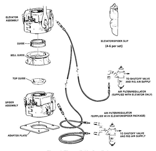
Figure 4: Elevator/Spider Installation
