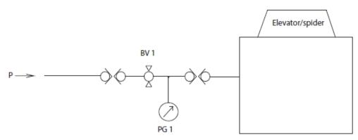
Figure 10: Pressure test schematic
