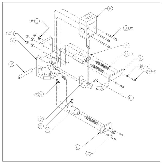
Figure 18: Valve & Latch Assembly
