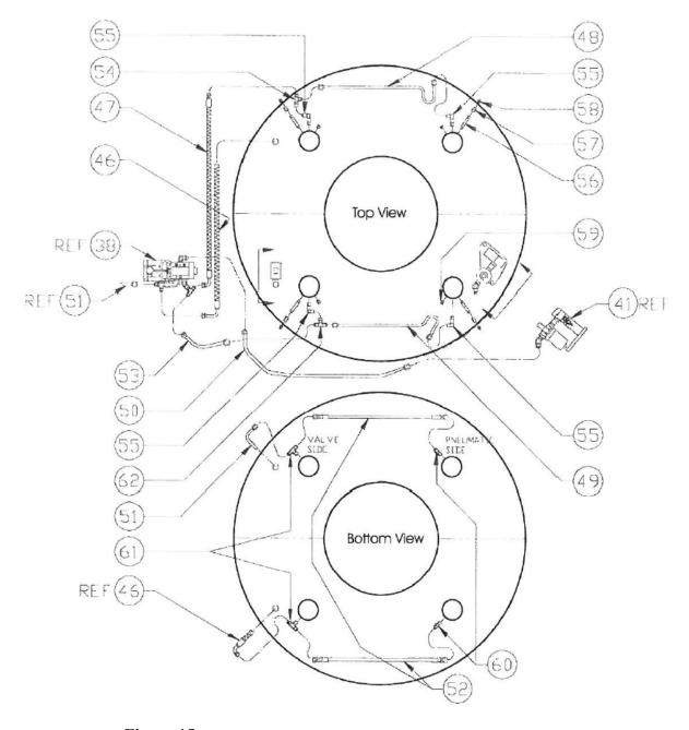
Figure 15: 750 Ton 14" Elevator/Spider Assembly (Part 2 of 2)
