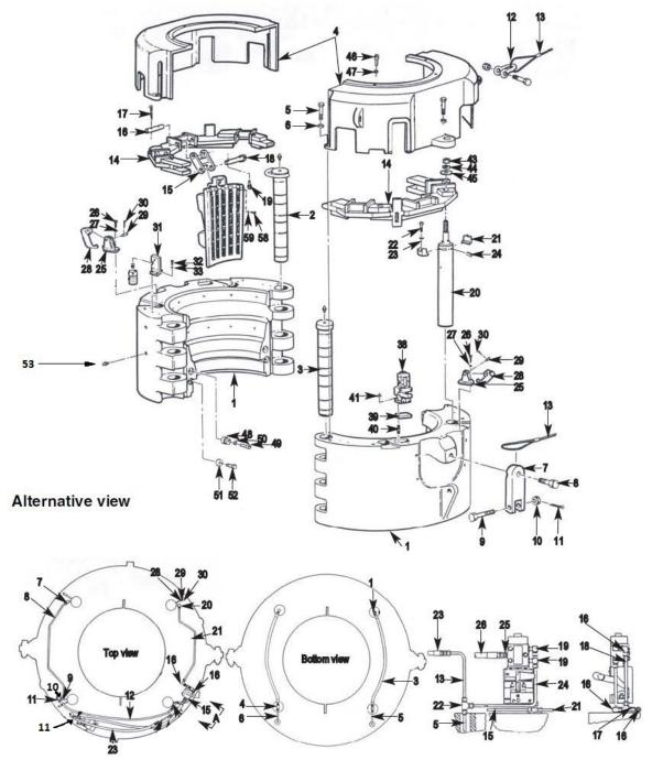
Figure 16: 750 Ton 24.5" Elevator/Spider Assembly
