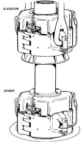
Figure 1: Elevator and Spider (500 ton unit shown)
