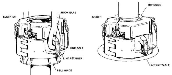
Figure 3: Elevator (Left) and Spider (Right) installed
