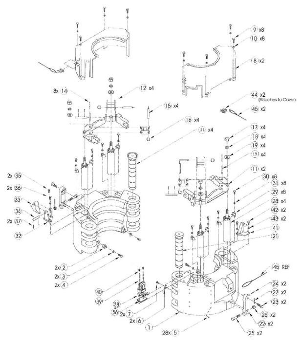
Figure 14: 750 Ton 14 / 24.5" Elevator/Spider Assembly (Part 1 of 2)
